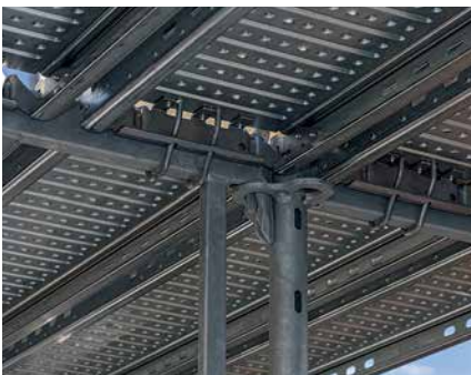
The protection against lifting is integrated in the decking: the securing device reaches around the ledger and secures the individual deck each time.
