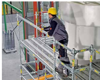
The Gravity Lock allows quick and safe assembly with site personnel always in a secure position, whereby the wedge drops into the rosette opening due to its own weight.
